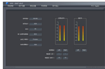
Web server monitoring the status of video and audio signal, the audio PPM before and after loudness control
